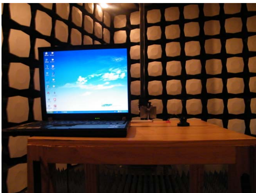
Picture 2: Radiated Spurious Emissions Test setup
