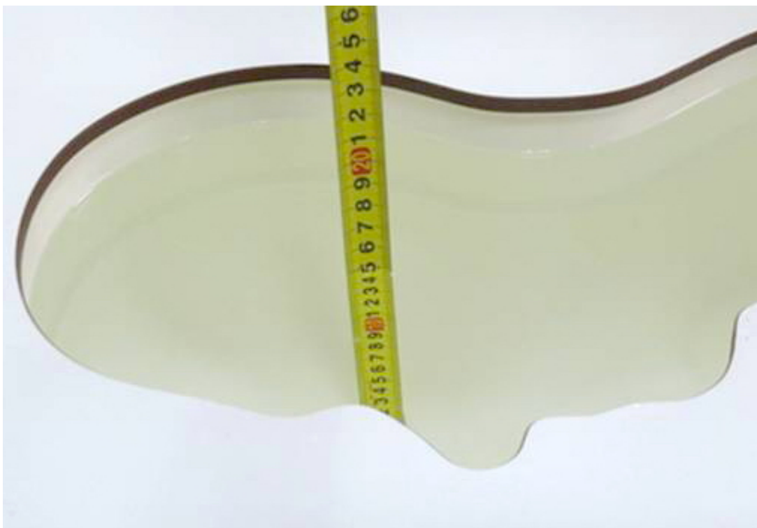
Picture 5: liquid depth in the head Phantom (1750 MHz, 15.1cm depth)
