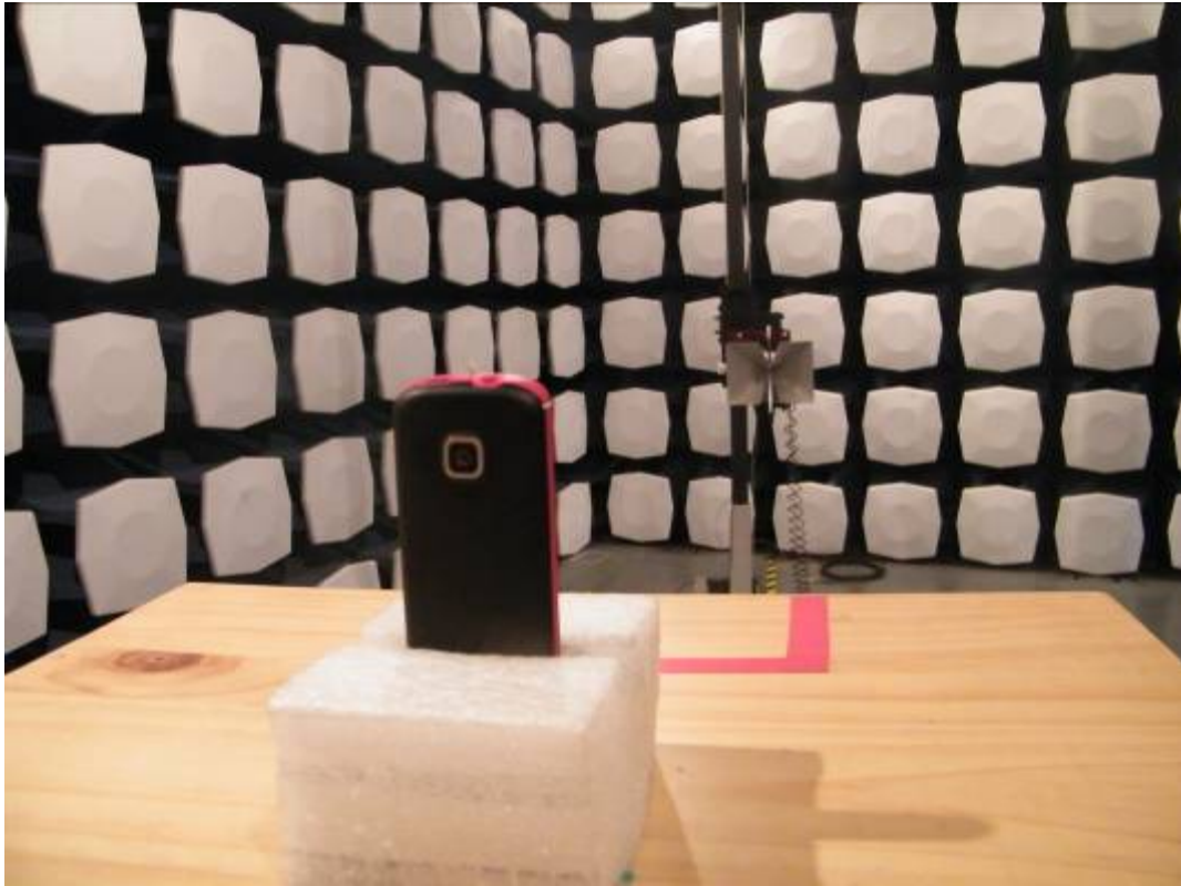
Picture 2: Radiated Spurious Emissions Test setup
