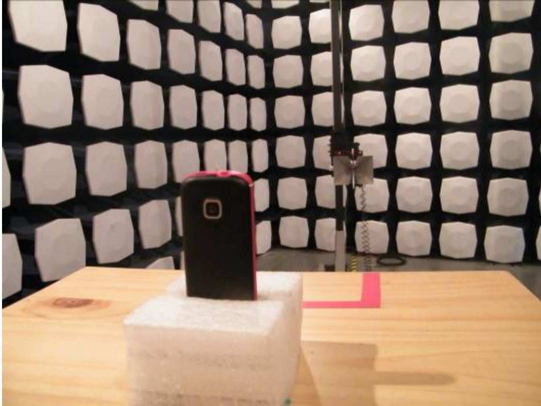
Picture 2: Radiated Spurious Emissions Test setup
