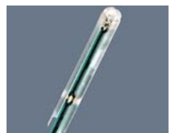
Figure 3 H3DV6 H-field Probe
