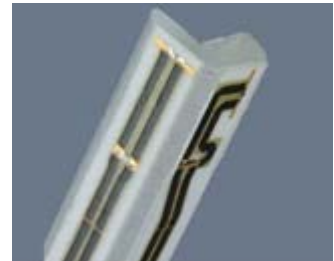
Figure 2 ER3DV6 E-field Probe
