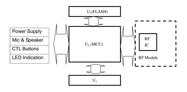
1. Applied IC in product, total 4 IC are applied in the product. They are  $U_1$ ,  $U_2$ ,  $U_3$ , and Radio Frequency(RF) IC in RF Module
