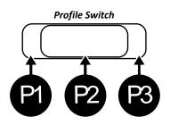
The Power Racer 270 can be set to one of three pre-set profiles allowing you to change the configuration of the wheel without the need to connect the wheel to a computer. Each of the profiles are selected using the Profile Switch, which can be set to the position 'P1', 'P2' and 'P3' representing each of the profiles as shown. The position of the Profile Switch can be changed at anytime with the wheel connected or disconnected from the console.
