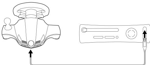
Connect the larger end of the USB Data/Charge Cable (supplied) into any free USB port on your Xbox 360.
