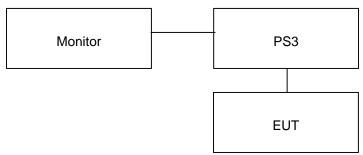
( $EUT \colon EVO^{TM}$  Wireless Controller for use with PS3  $_{\circledR})$
