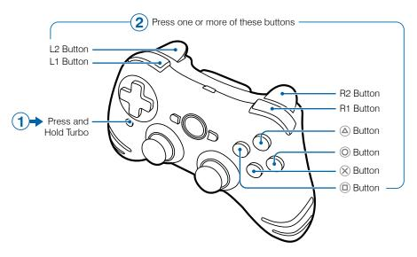
The TurboFire Wireless Controller will remember this configuration until the batteries become flat or are removed or the process is repeated to configure a different set of buttons.
