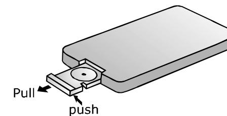
\* Press the tab on the underside of the battery cover and at the same time pull out the battery tray.
