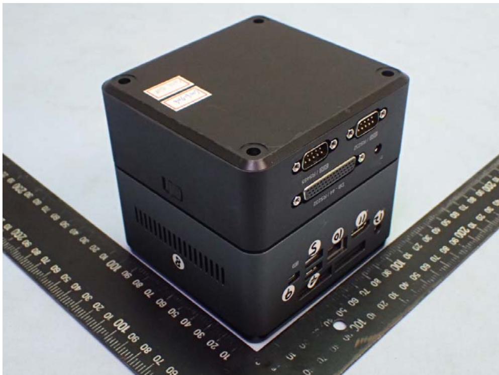
Figure 8 Personal Computer (SKM-U mPC) with COM Box, General Appearance (Front & Side View)
