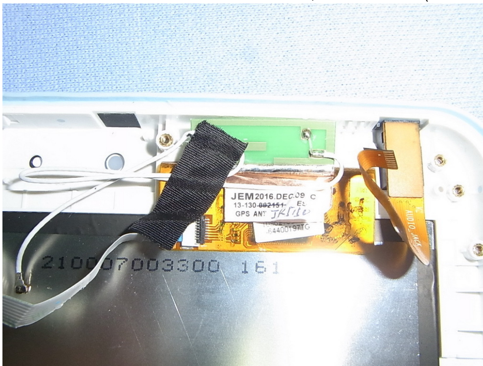
Figure 46 7" Multi Function Pad, Internal View (GPS Antenna)
