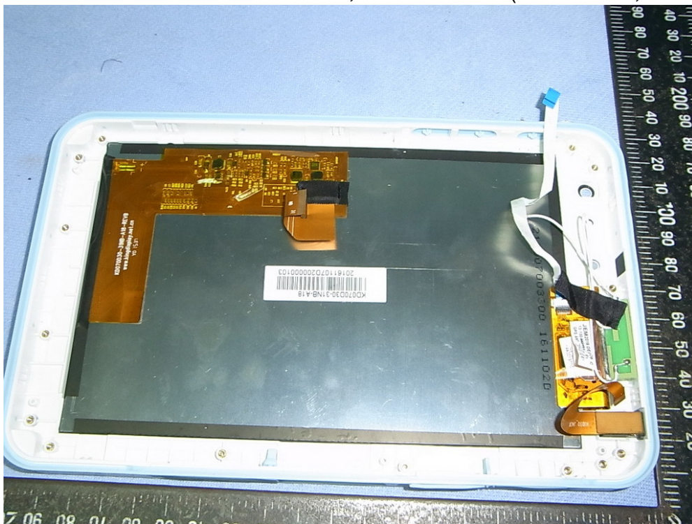
Figure 48 7" Multi Function Pad, Internal View (LCD Panel, Label View)
