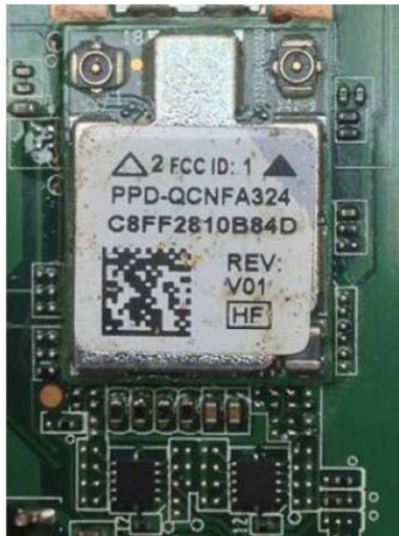
Figure 36 7" Multi Function Pad, Internal View (Wireless Module)
