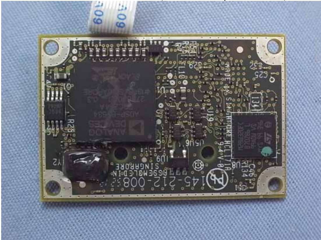
Figure 37 7" Pocketable Pad, Internal View (Control Board, Front View)
