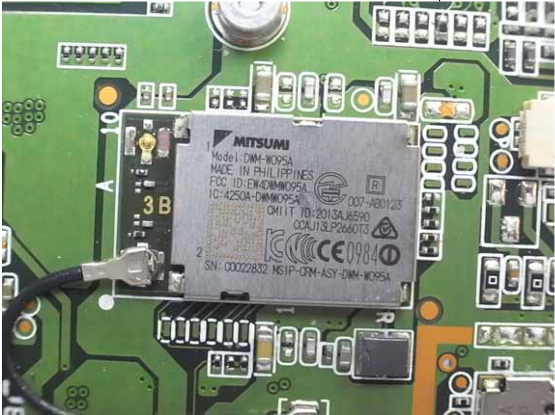
Figure 39 7" Pocketable Pad, Internal View (WLAN+BT Module)
