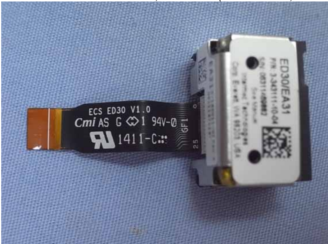
Figure 32 7" Pocketable Pad, Internal View (Barcode Scanner, Front View)
