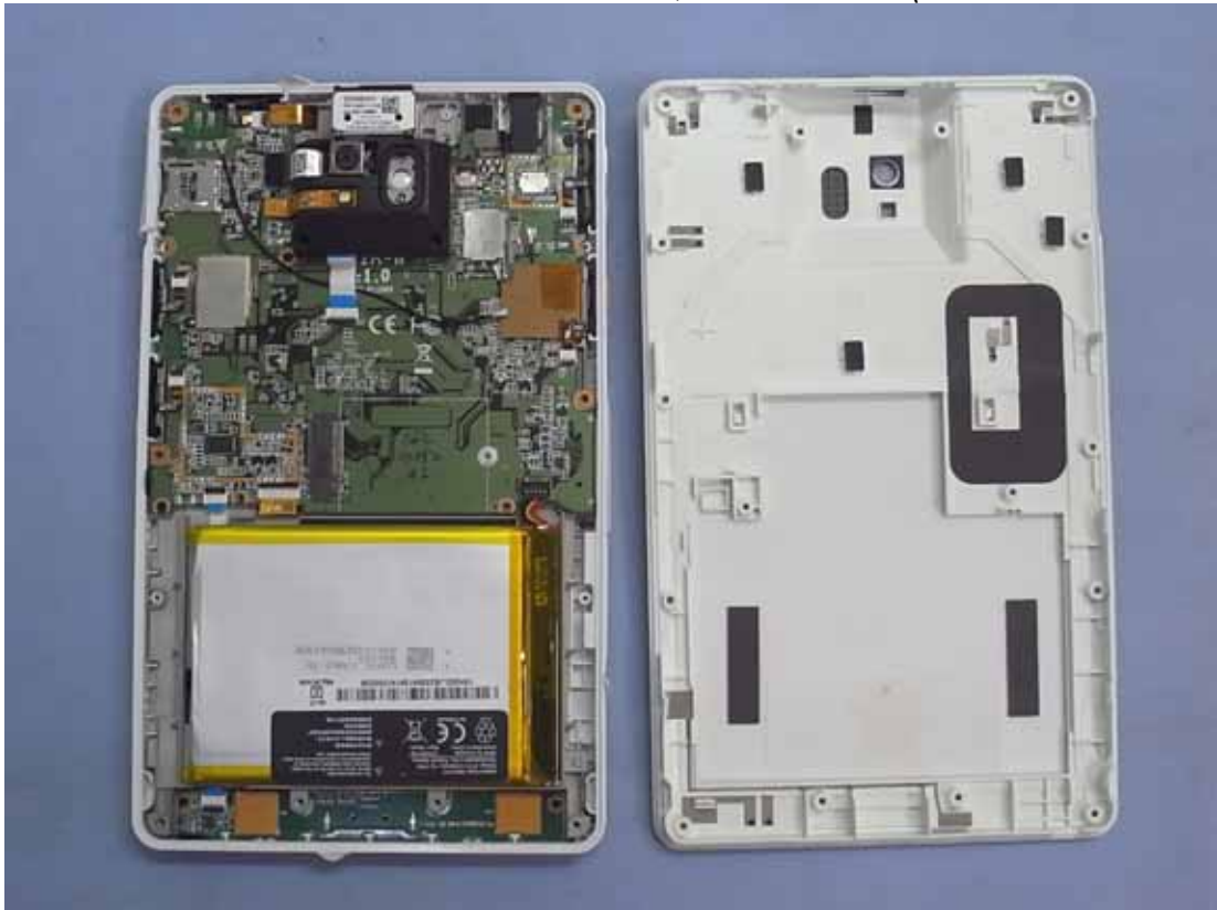
7" Pocketable Pad, Internal View (Removed Back Cover)
