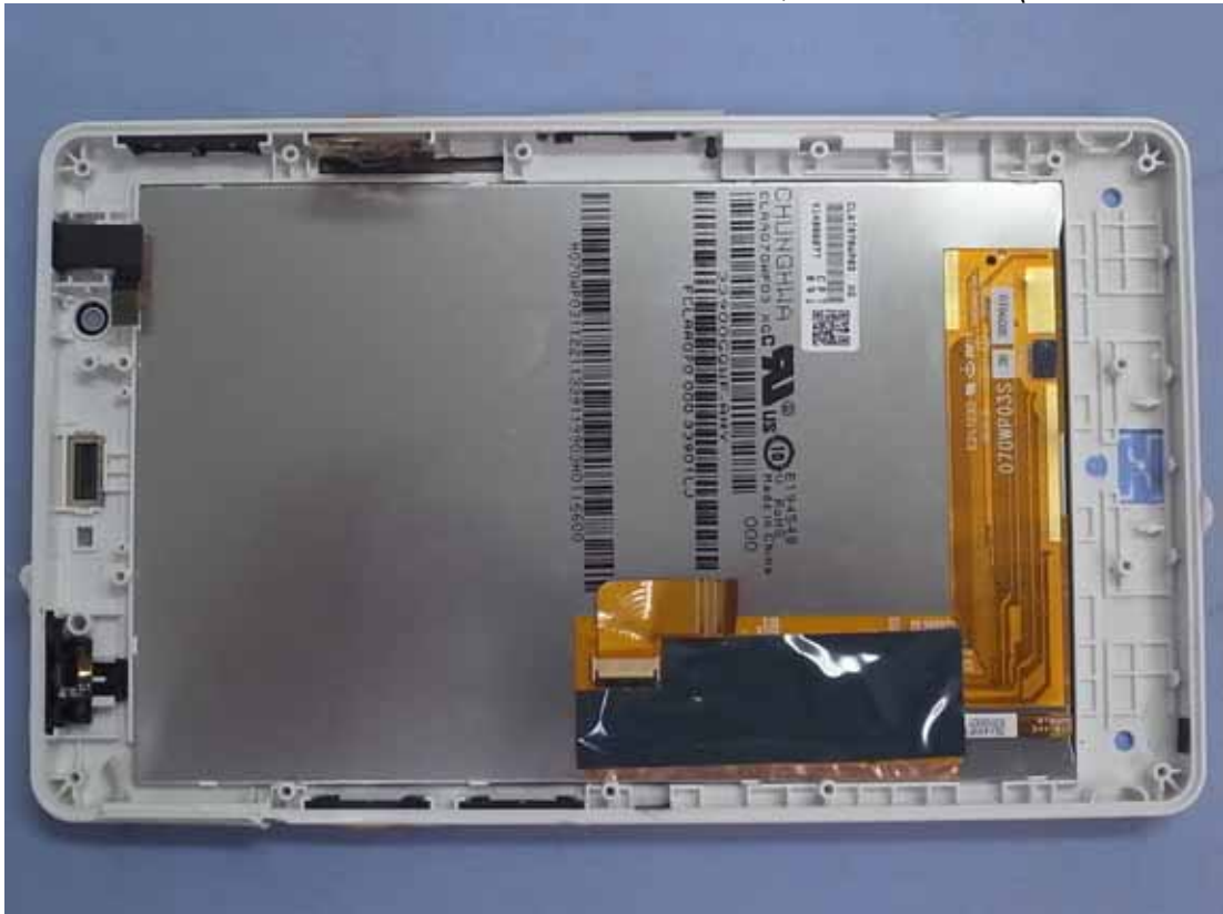
Figure 51 7" Pocketable Pad, Internal View (Frame of Panel)
