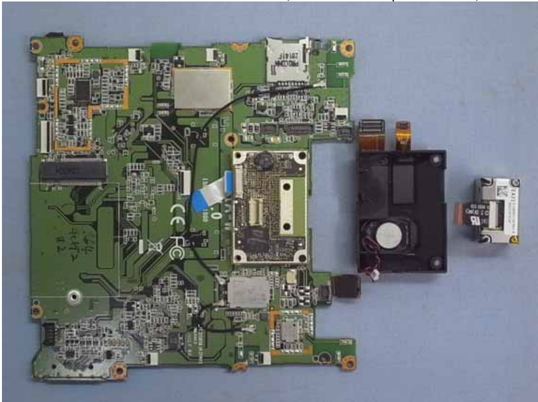
Figure 31 7" Pocketable Pad, Internal View (Main Board, Front View)
