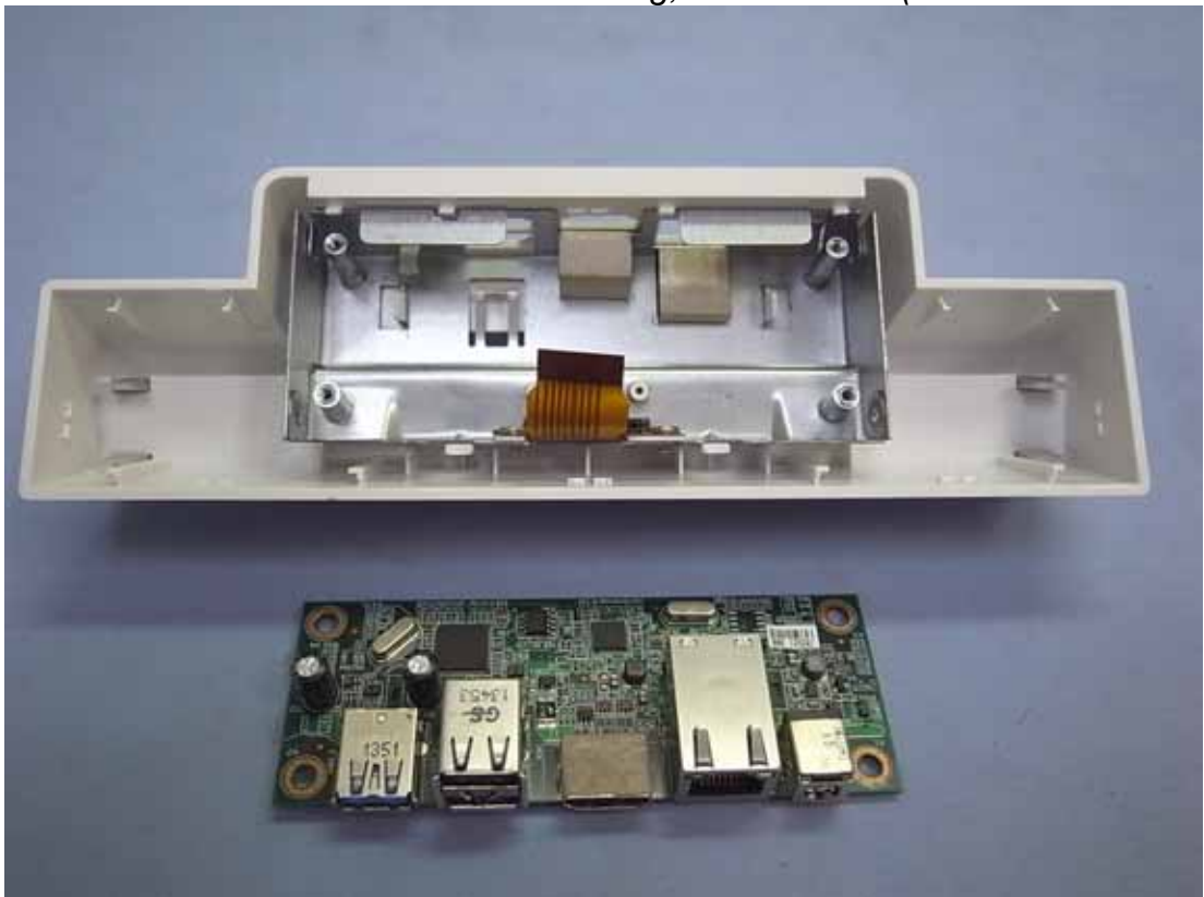
Figure 57 Docking, Internal View (Main Board, Front View)
