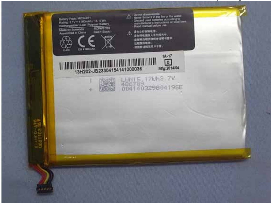
7" Pocketable Pad, Internal View (Battery Pack View)
