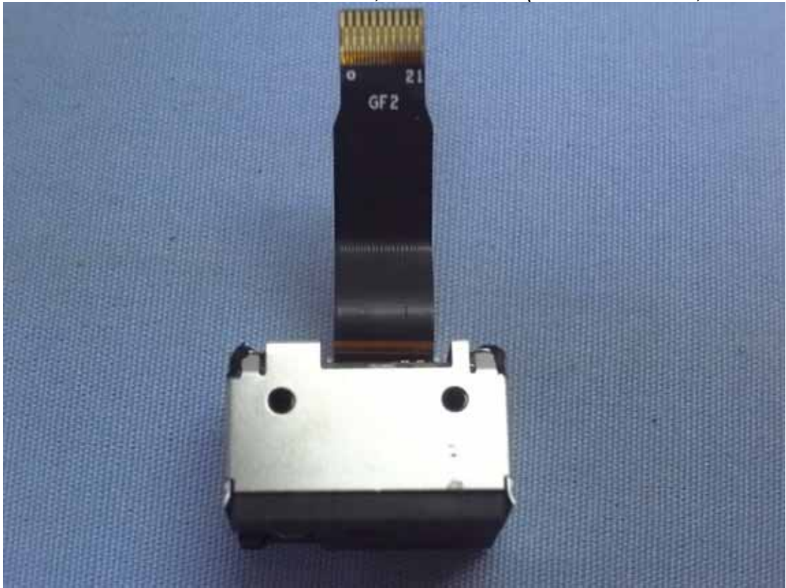
Figure 33 7" Pocketable Pad, Internal View (Barcode Scanner, Back View)
