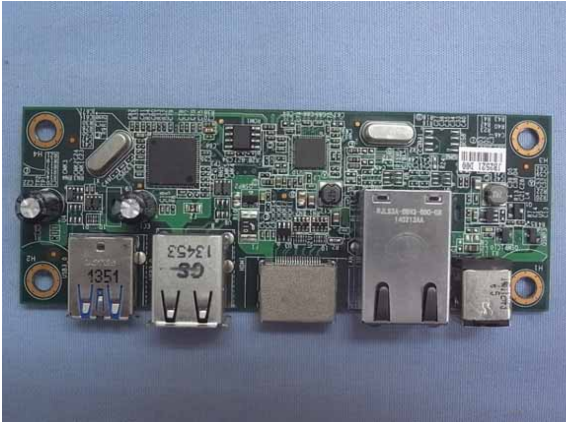
Figure 58 Docking, Internal View (Main Board, Back View)
