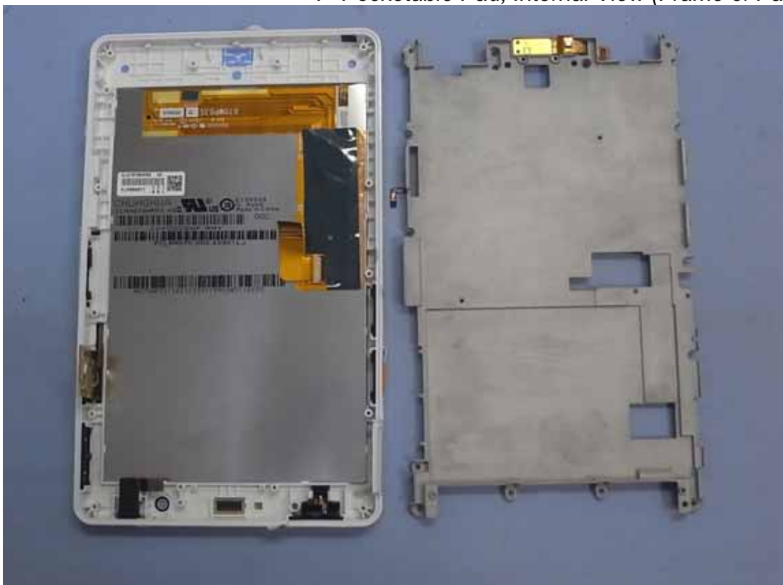
Figure 50 7" Pocketable Pad, Internal View (Frame of Panel)
