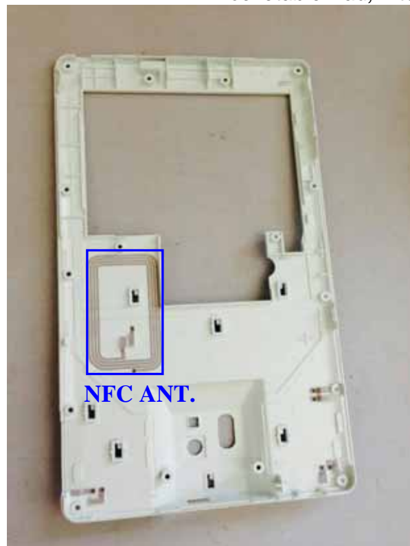
Figure 54 7" Pocketable Pad, Internal View (Antenna View)
