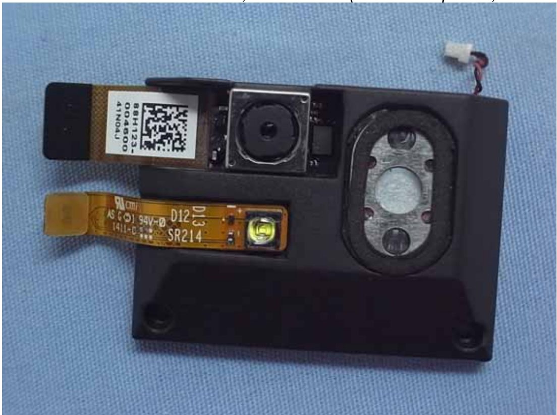
Figure 34 7" Pocketable Pad, Internal View (Camera & Speaker, Front View)
