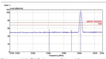
Audix NO.1 Chamber 3m 3115(4927) ABOVE 1GHZ(PK) 28\*C / 43% N9010A TB71A-H Site no. Dis. / Ant. Limit Env. / Ins. EUT Power Rating : DC5V Test Mode : Out of band SDPSK
