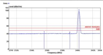
: Audix NO.1 Chamber :3m 3115(4927) :ABOVE 1GHZ(AV) :20=C / 43% N9010A :TB71A-H :DC5V Site no. Dis. / Ant. Limit / Ins.
