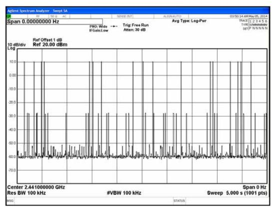
7.6.6. Type of Modulation: GFSK, Test Frequency: 2480MHz
