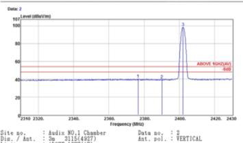
Audix NO.1 Chamber 3m 3115(4927) ABOVE 1GHZ(AV) 28\*C / 43% N9010A TB71A-H DC5V Site no. Dis. / Ant. Limit
