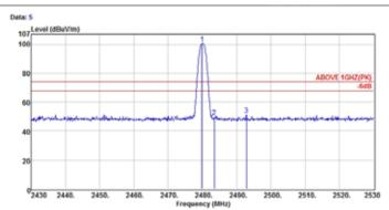
Remarks: 1. Emission Level: Antenna Factor + Cable Loss + Reading 2. The emission levels that are 20dB below the official limit are not reported.
