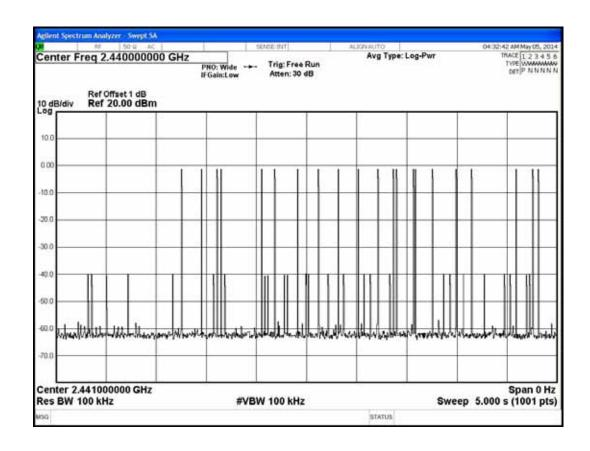
7.6.3. Type of Modulation: 8-DPSK, Test Frequency: 2480MHz
