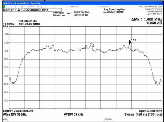
Test Mode: 8-DPSK, 2480MHz adjacent channel of carrier frequency separation
