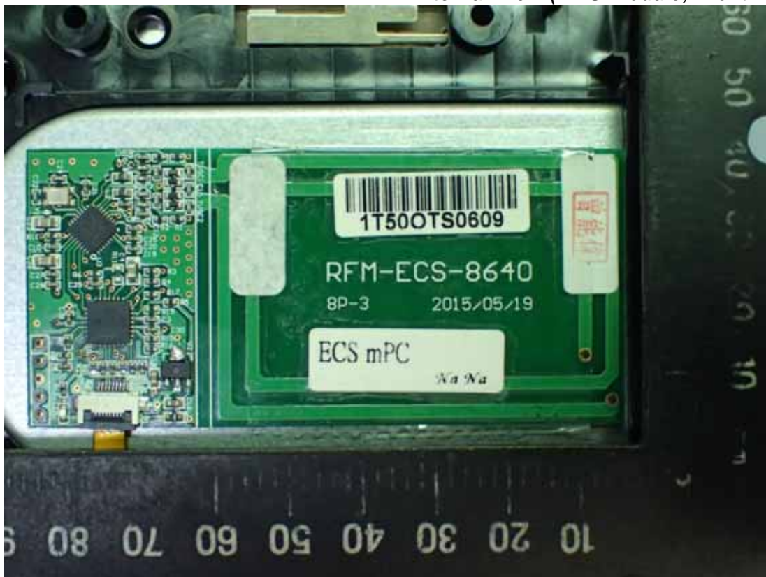
Figure 32 Internal View (NFC Module, Front View)
