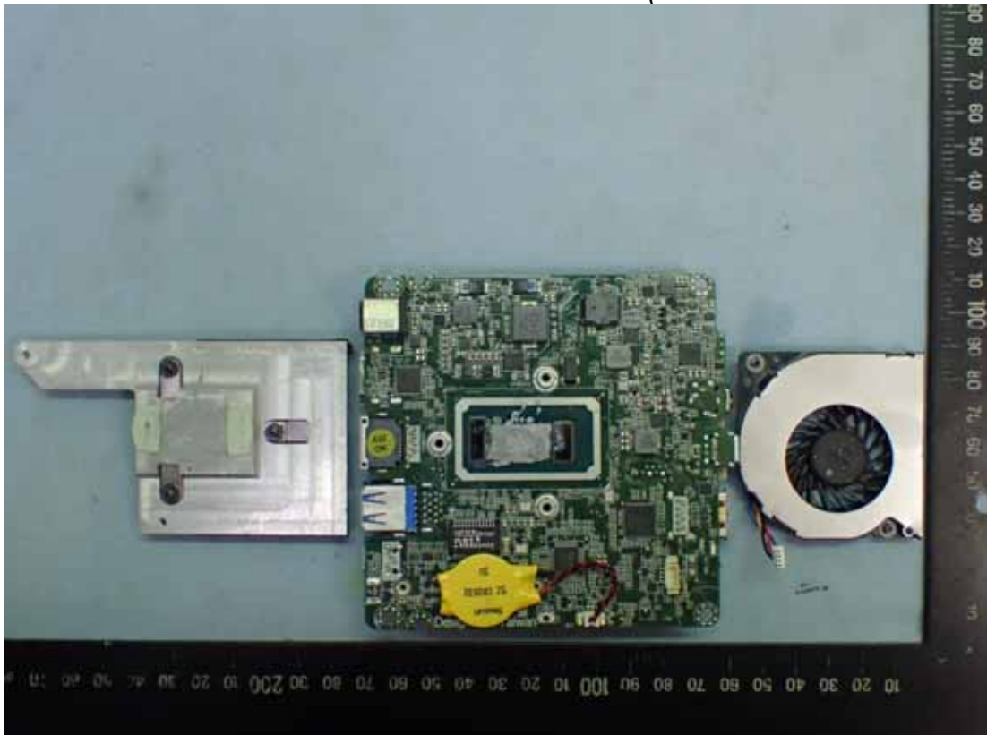
Figure 21 Internal View (Removed Heat-Sink and Fan)
