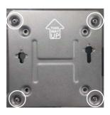
2. Fasten 2 screws under the case.
