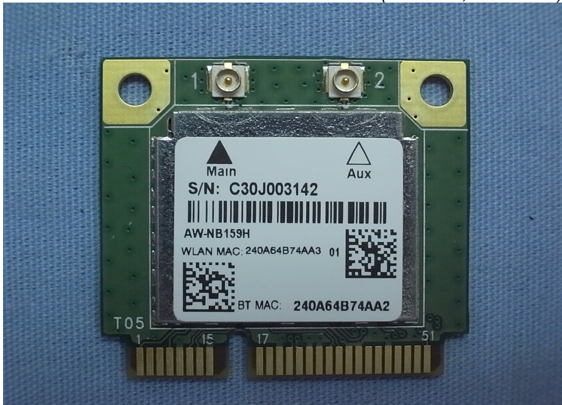
Figure 9 Internal View (RF Board, Front View)
