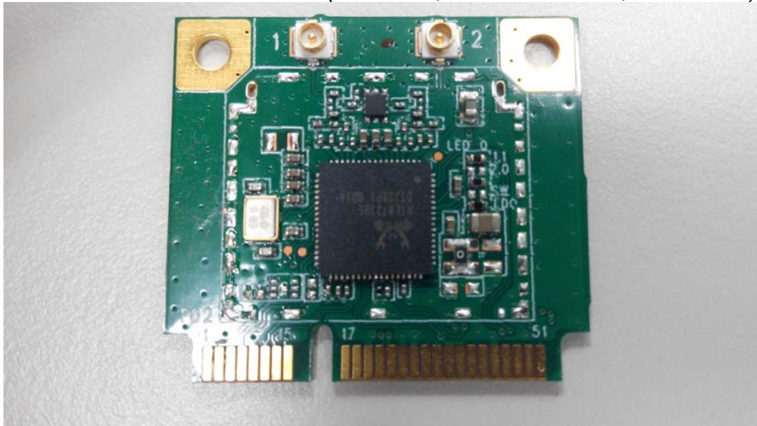
Figure 11 Internal View (RF Board, Removed Cover, Front View)
