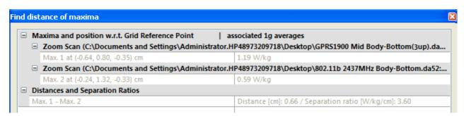
Result: The SAR to peak location separation ratio is less than 0.04, so simultaneous transmission is not applicable.
