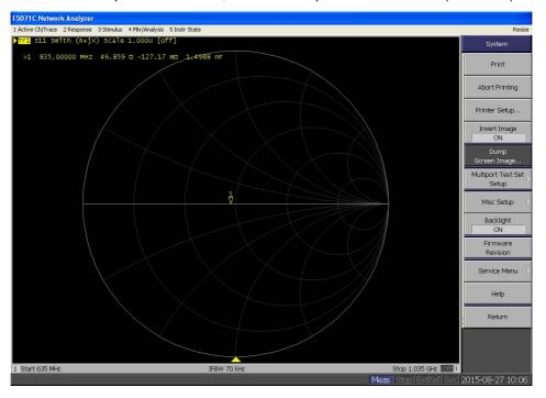
Calibrated return loss: -24.3 dB; Measured return loss: -25.239dB (within 20%)
