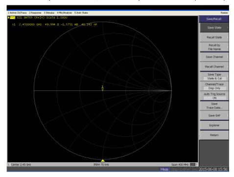
Calibrated return loss: -26.2 dB; Measured return loss: -25.169dB (within 20%)
