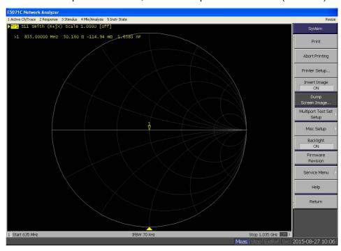
Calibrated return loss: -30.2 dB; Measured return loss: -29.523dB (within 20%)
