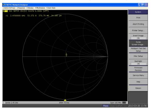
Calibrated return loss: -27.363 dB; Measured impedance: -28.403 dB (within 20%)
