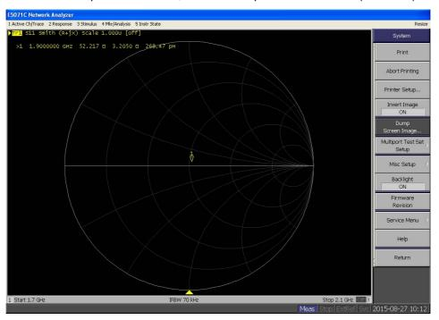
Calibrated return loss: -23.6 dB; Measured return loss: -24.035dB (within 20%)
