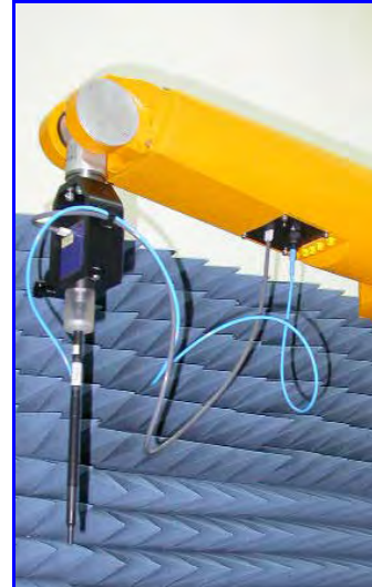
Figure 4. Probe setup on robot
