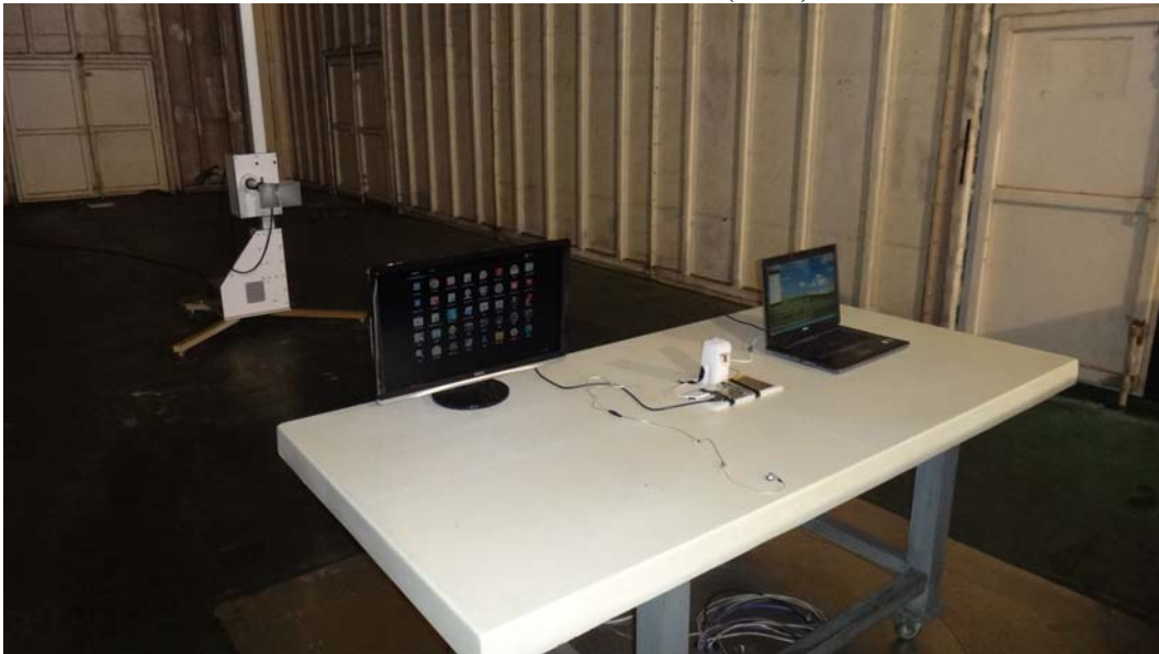
Front View of Radiated Test (Horn)
