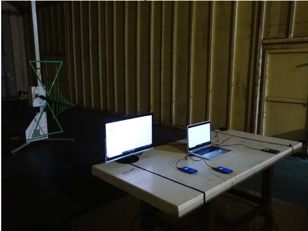
Front View of Spurious Emission Test
