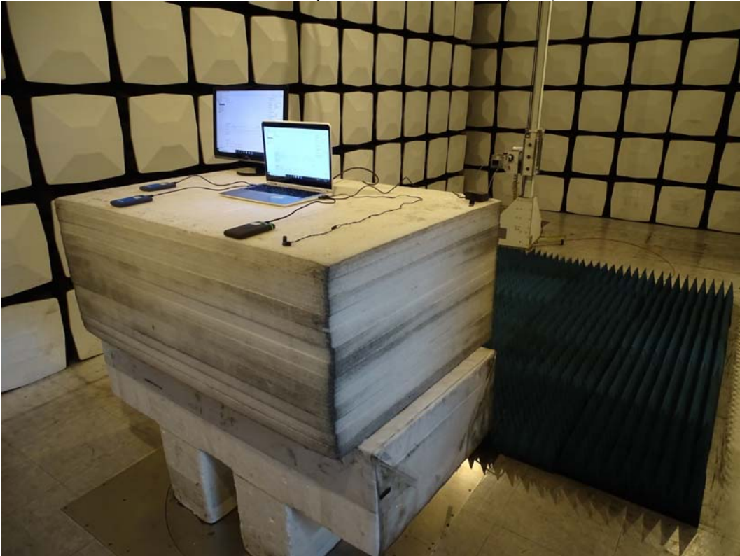
Front View of Spurious Emission Test (Horn)
