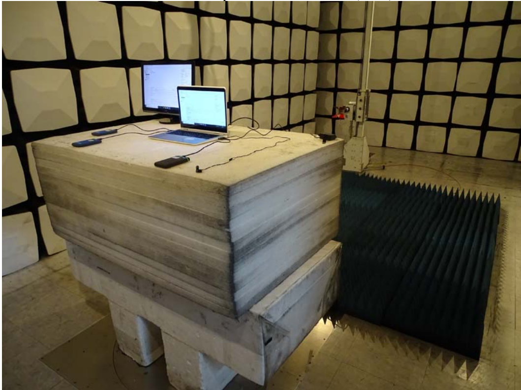
Front View of Spurious Emission Test (Horn)
