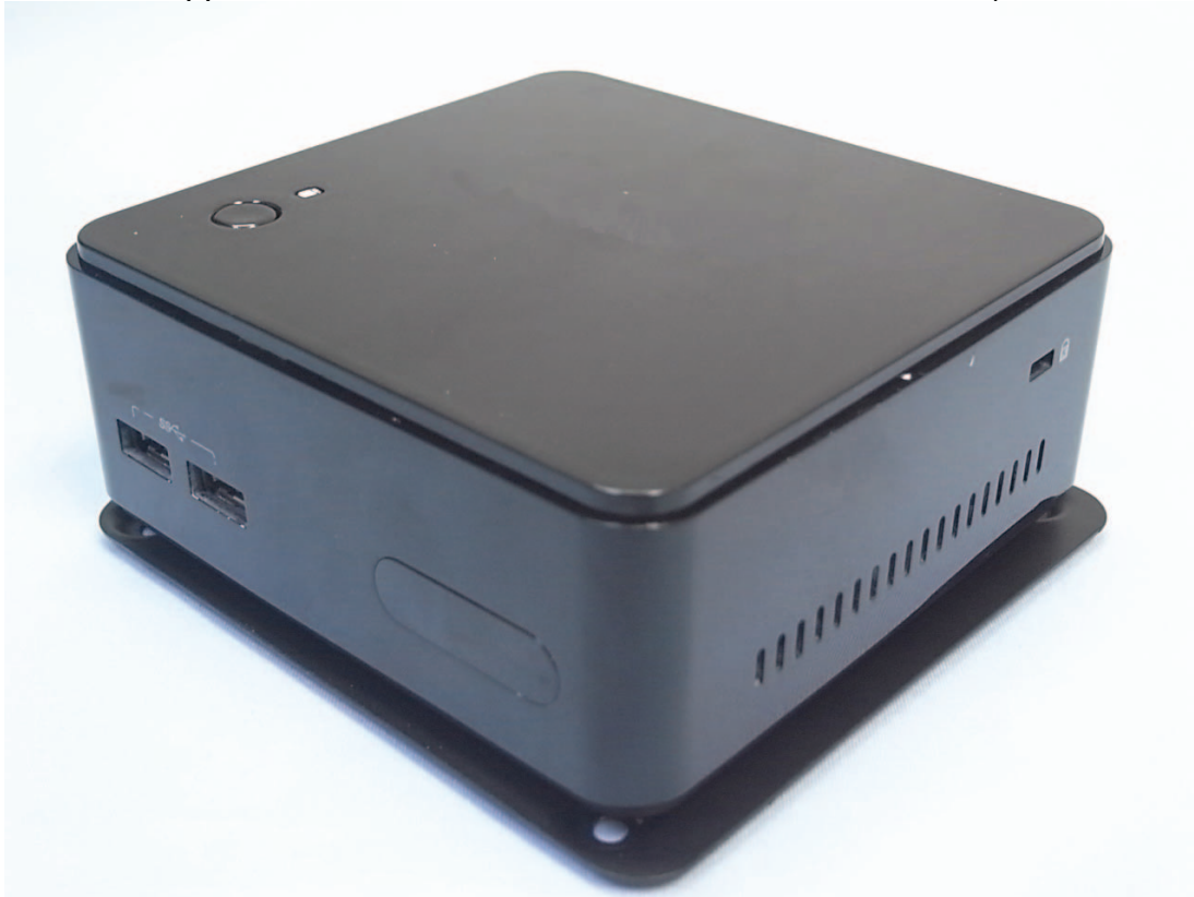
Figure 3 General Appearance w/Metal Case and VESA Mount Bracket (Front and Side View)
