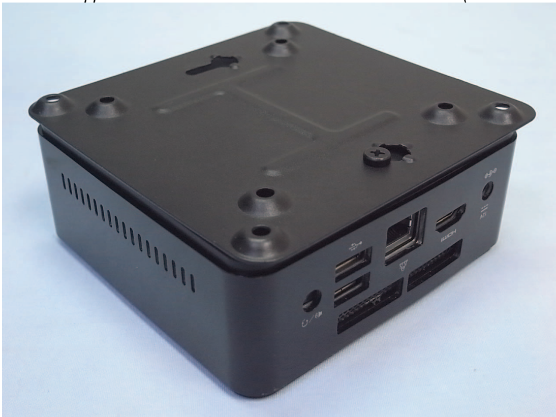
Figure 4 General Appearance w/ Metal Case and VESA Mount Bracket (Back and Side View)
