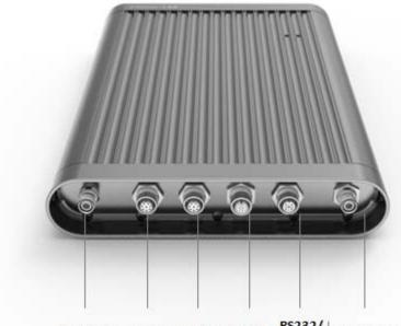
Antenna⊬ DC-IN- USB2.0+ USB3.0+ RS232/↓ Antenna⊬ RS485+
