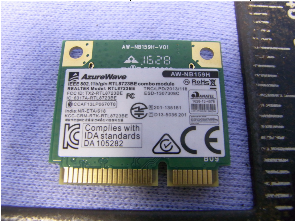
Figure 16 Internal View (Wi-Fi + BT Combo Module, Back View)
