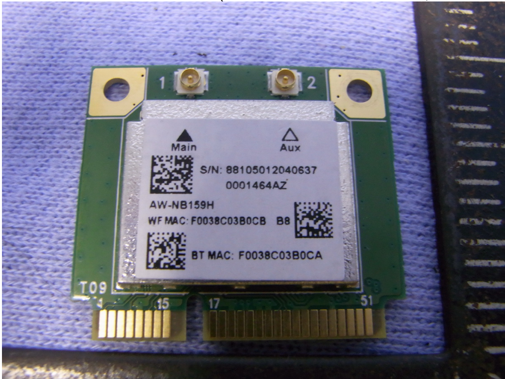
Figure 15 Internal View (Wi-Fi + BT Combo Module, Front View)
