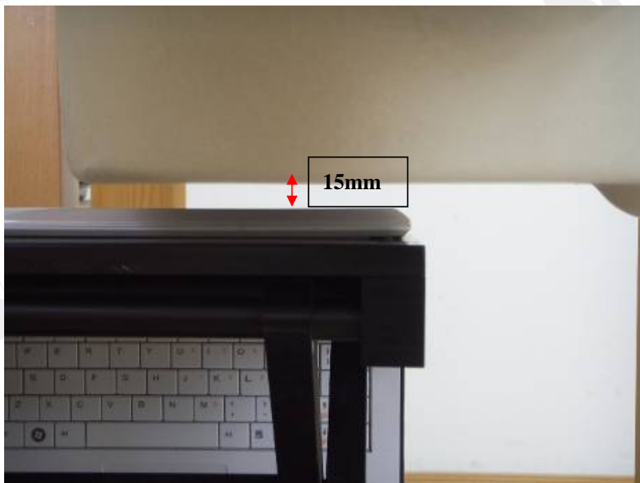
Fig.8 Back side of Notebook is paralleled with flat phantom, and spacing between EUT and Phantom is 15mm.
