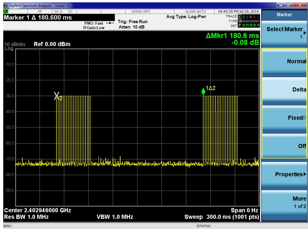
total 15 burst in 1 cycle, 180.6ms for 1cycle
