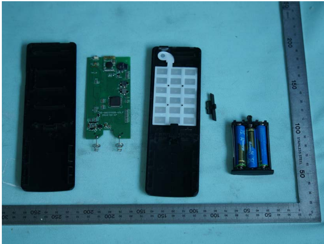
FIGURE 1 REMOTE CONTROLLER (M/N: SFD-Y-14) COVER REMOVED
