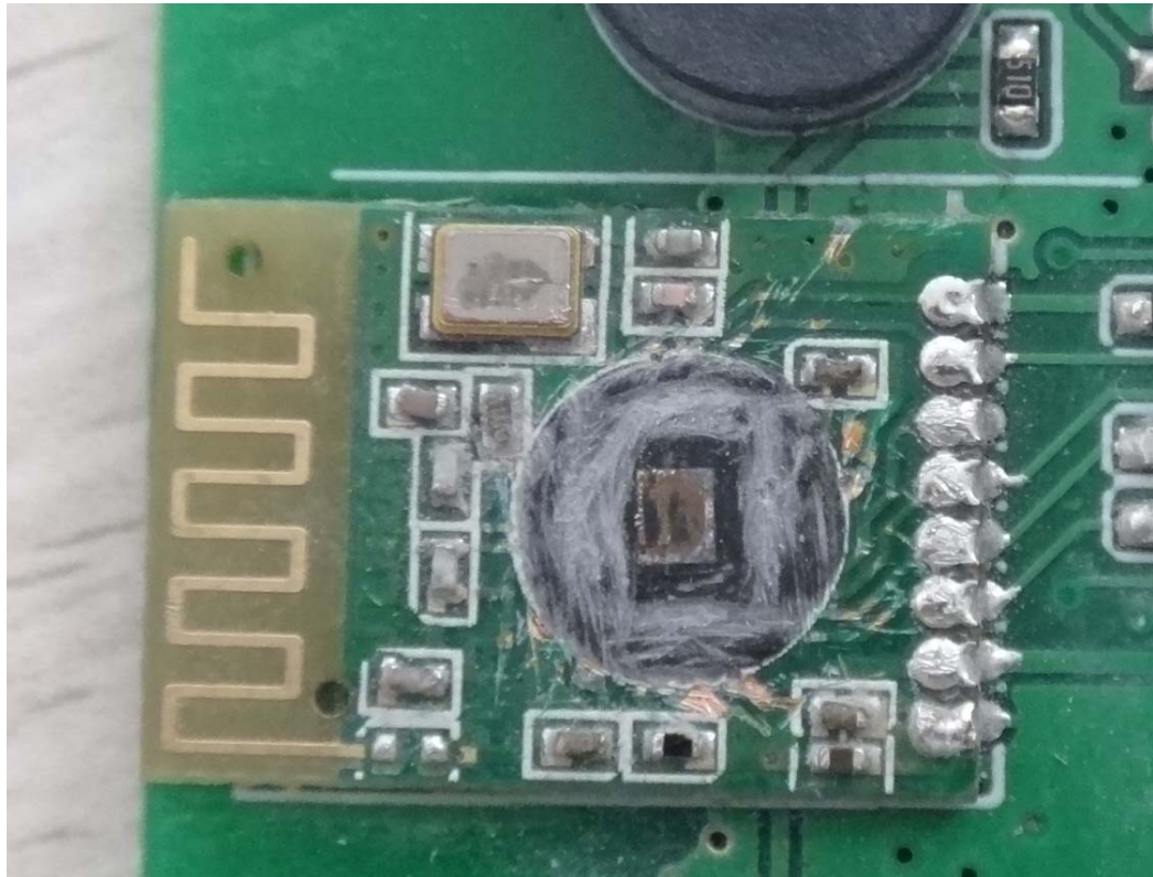
FIGURE 5 REMOTE CONTROLLER (M/N: SFD-Y-14) RF MODULE (CHIP RUBBER REMOVED)
