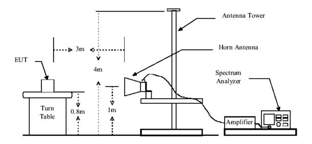
The field strength is calculated by adding the Antenna Factor, Cable Factor & preamplifier. The basic equation with a sample calculation is as follows:
