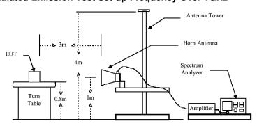
The field strength is calculated by adding the Antenna Factor, Cable Factor & preamplifier. The basic equation with a sample calculation is as follows:
