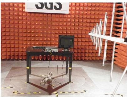
3. Radiated Spurious emission measurement(Above 1GHz)
