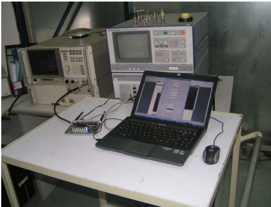
Conducted test for antenna port
