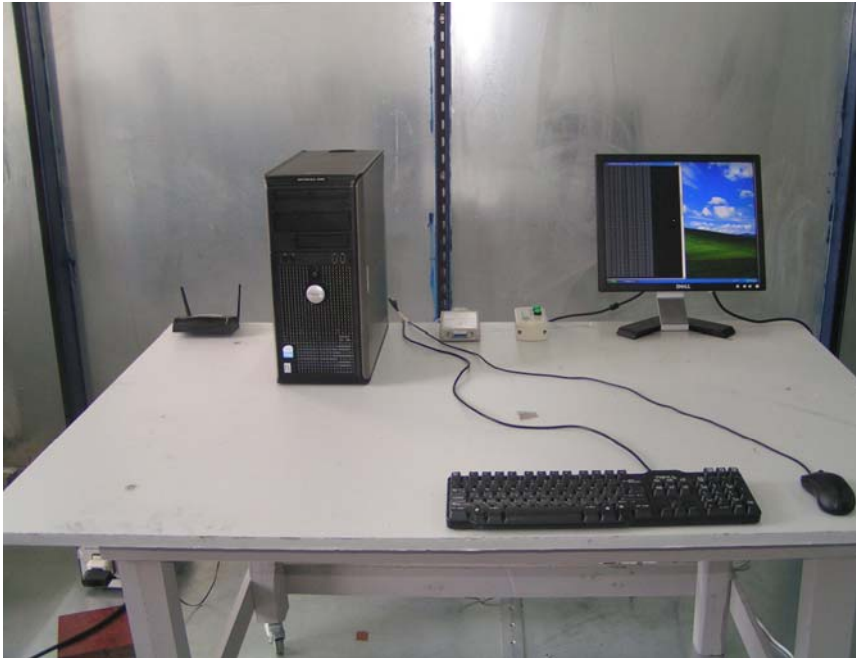
Conducted Emission Test Set-up View
