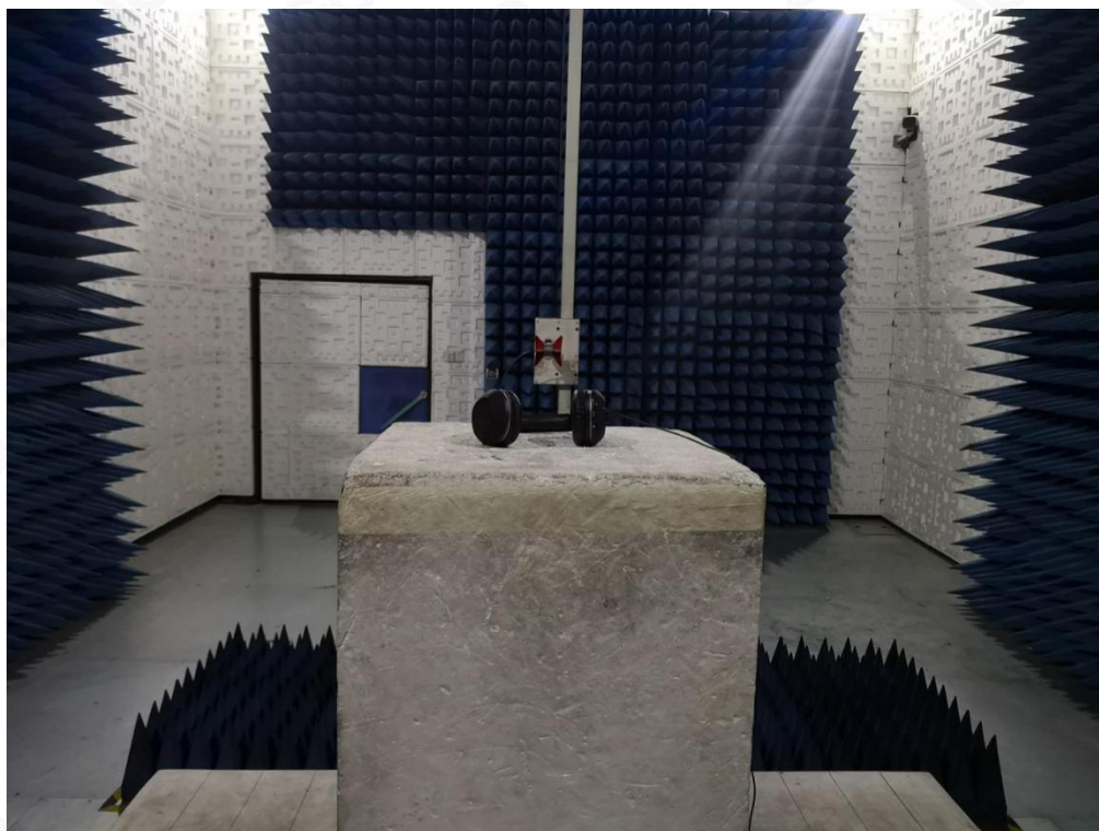
RADIATED EMISSION TEST SETUP ABOVE 1GHZ
