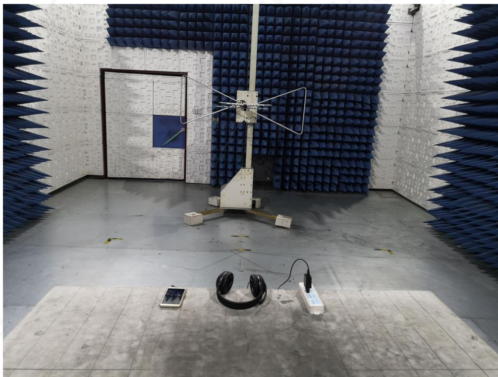
RADIATED EMISSION TEST SETUP ABOVE 1GHZ
