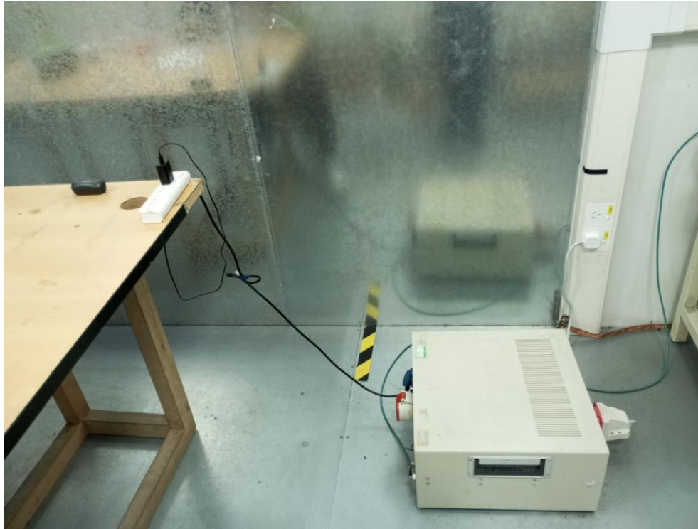
Conducted Emission Test Setup:
