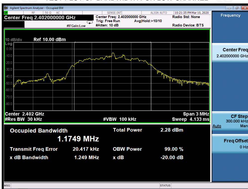
TEST PLOT OF BANDWIDTH FOR LOW CHANNEL
