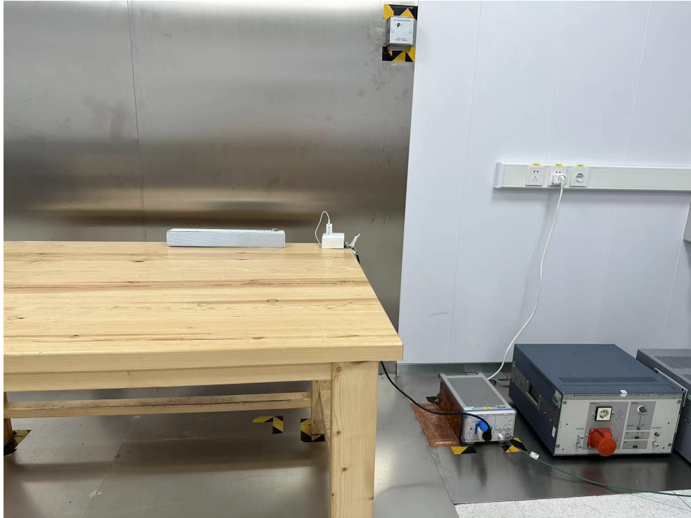
Radiated Emission Test View((Below 1G)
