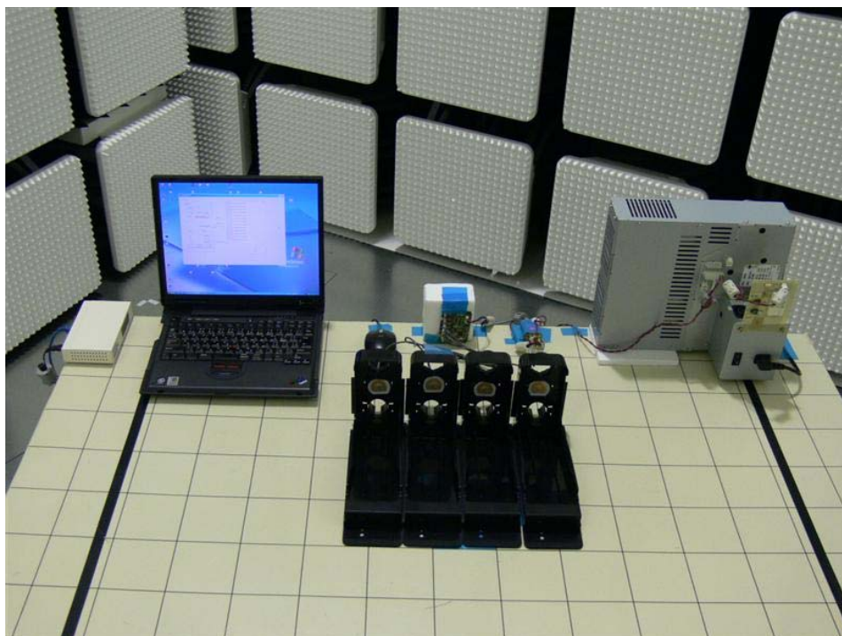
Photograph 10: Set-up for Radiated Emission, Close View
