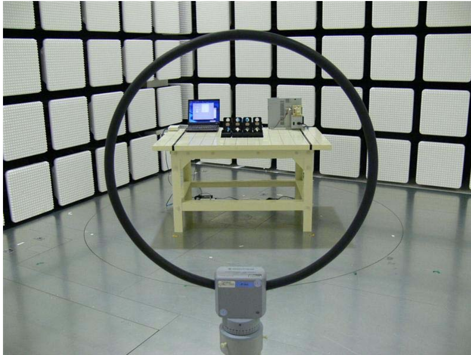
Photograph 9: Set-up for Radiated Emission, including Loop Antenna
