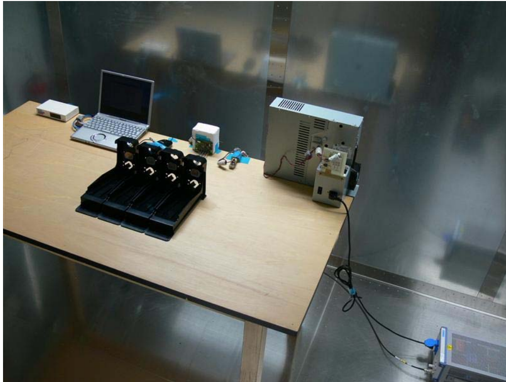
Photograph 7: Set-up for Conducted Emission, on AC Mains, Front View
