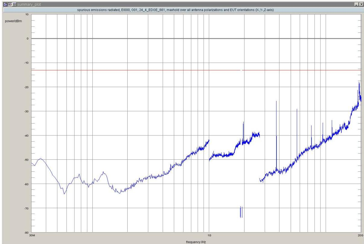
**Test: 24.4; Frequency Band = 1900, Mode = EDGE, Channel = 810, Frequency = 1909.8MHz**
