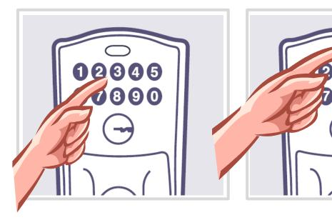
Enter the six digit program code. Wait for the Schlage button to flash and beep three times. Press the Schlage button and then the number 0. The hub will beep once it has found the lock.
