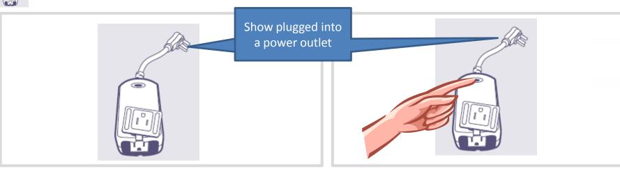
Plug the Outdoor module into an outlet that is no more than 10 foot from your Smart Hub.
