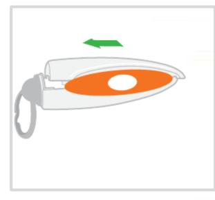
Lever open the key fob using the supplied tool.
