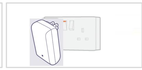
Plug the range extender into an outlet that is no more than 10 foot from your smart hub.
