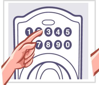
Enter the six digit program code. Wait for the Schlage button to flash and beep three times.
