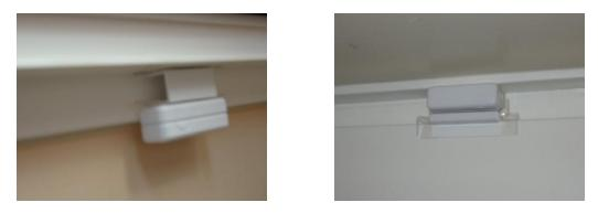
These images also show the use of a bit of electrical cable conduit, such as can be obtained from DIY stores, to move the main part of the sensor away from the door frame itself.
