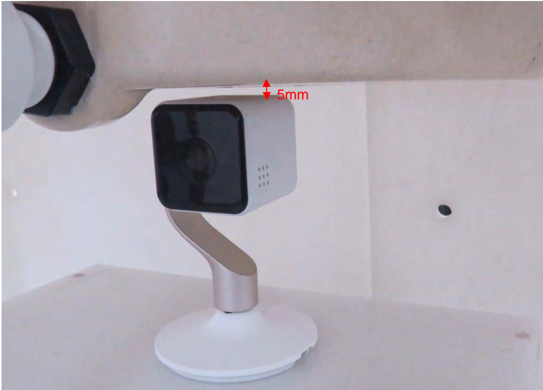
Picture 12: Top Side, the distance from EUT to the bottom of the Phantom is 5mm
