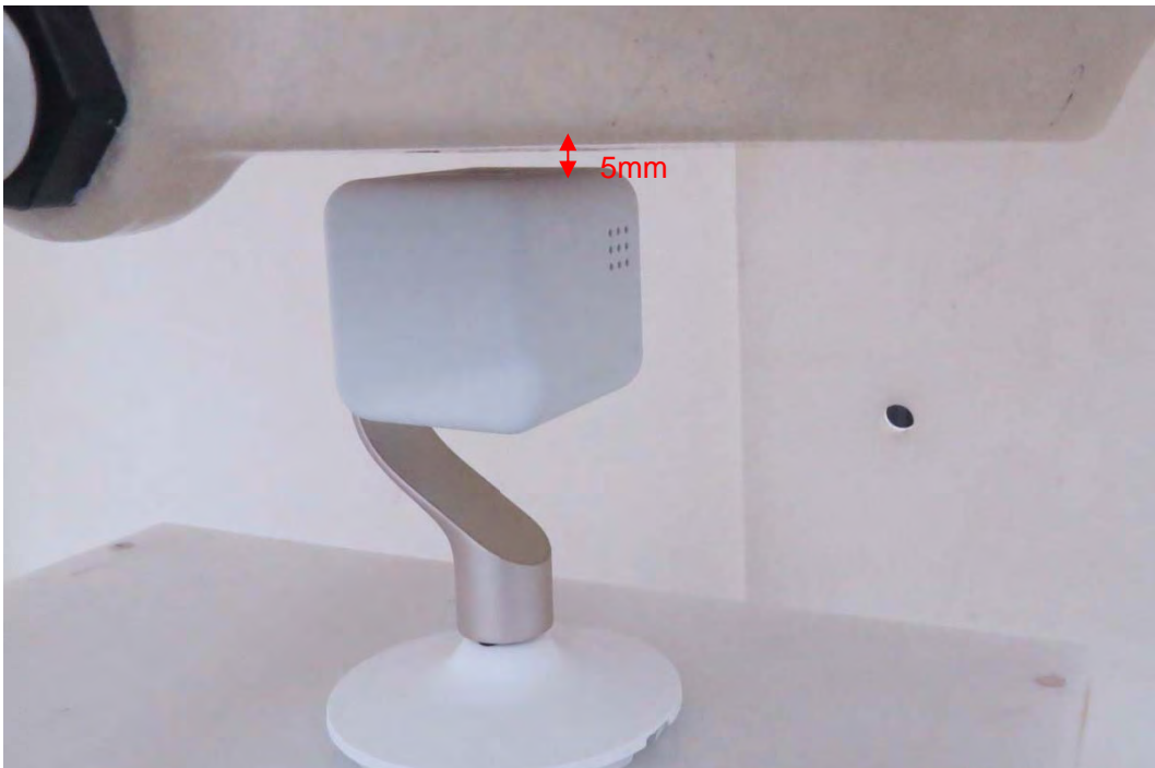
Picture 13: Bottom Side, the distance from EUT to the bottom of the Phantom is 5mm
