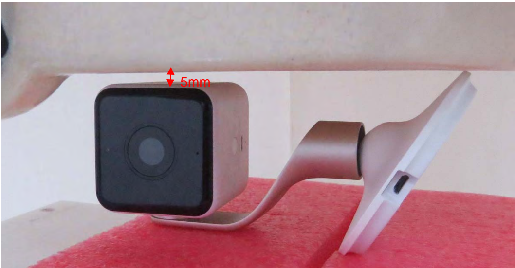
Picture 11: Right Side, the distance from EUT to the bottom of the Phantom is 5mm
