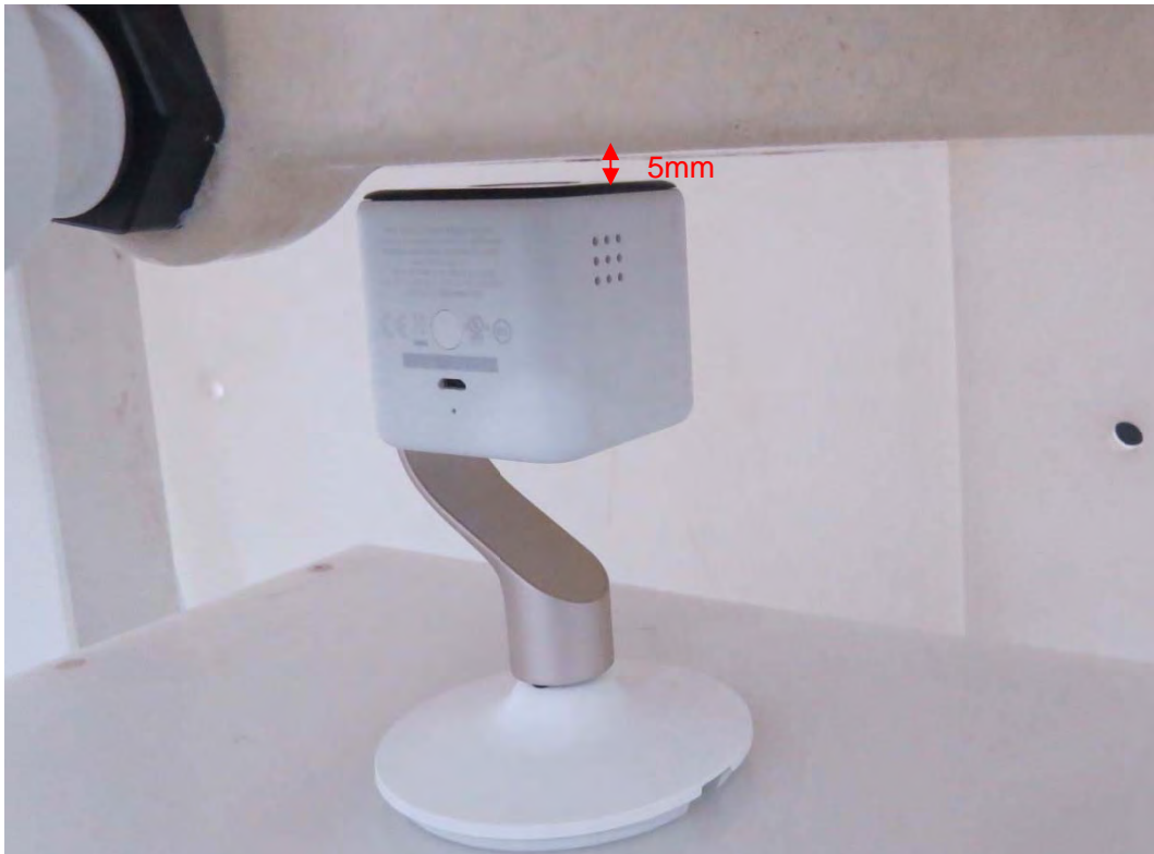
Picture 9: Front Side, the distance from EUT to the bottom of the Phantom is 5mm
