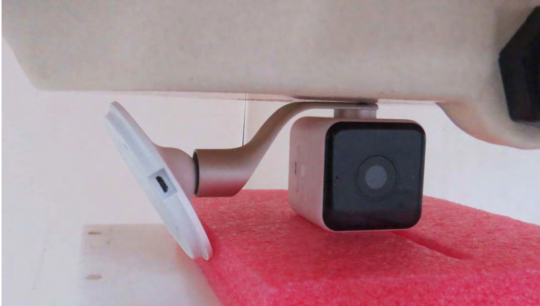
Picture 10: Left Side, the distance from EUT to the bottom of the Phantom is 0mm
