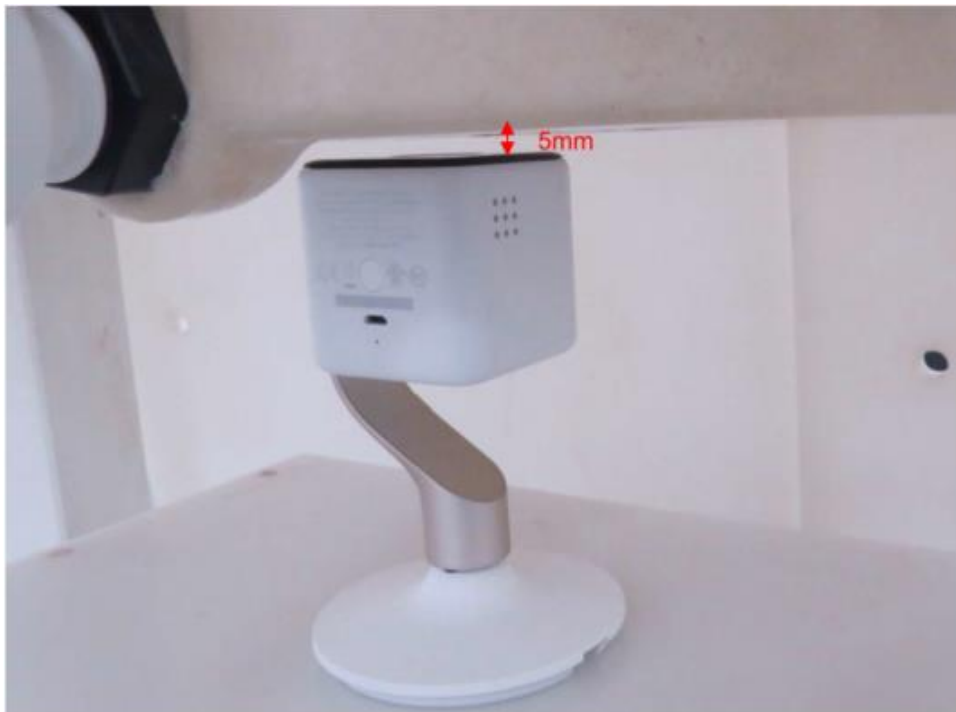
Front side, the distance from EUT to the bottom of the Phantom is 5mm
