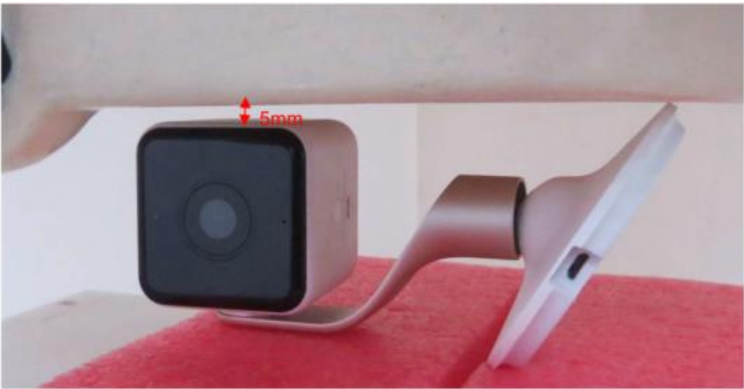
Right side, the distance from EUT to the bottom of the Phantom is 5mm
