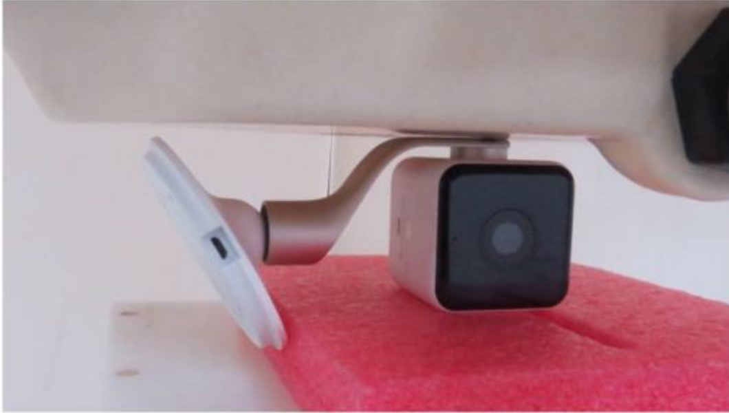
Left side, the distance from EUT to the bottom of the Phantom is 5mm
