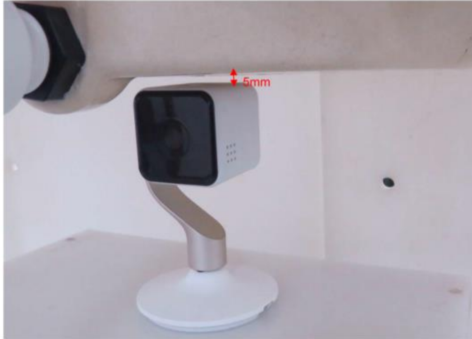
Top side, the distance from EUT to the bottom of the Phantom is 5mm
