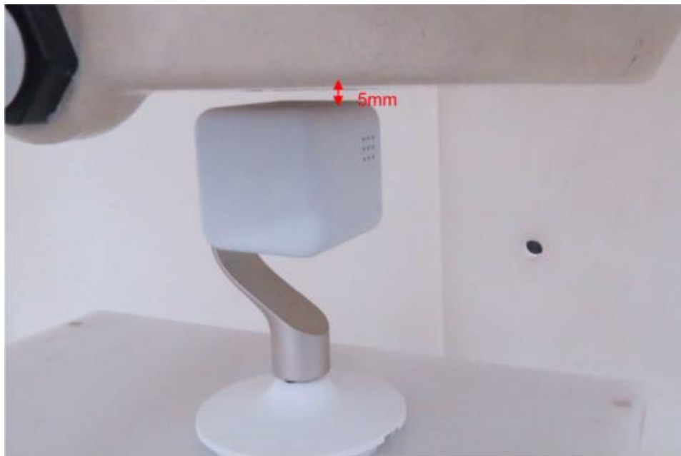
Bottom side, the distance from EUT to the bottom of the Phantom is 5mm
