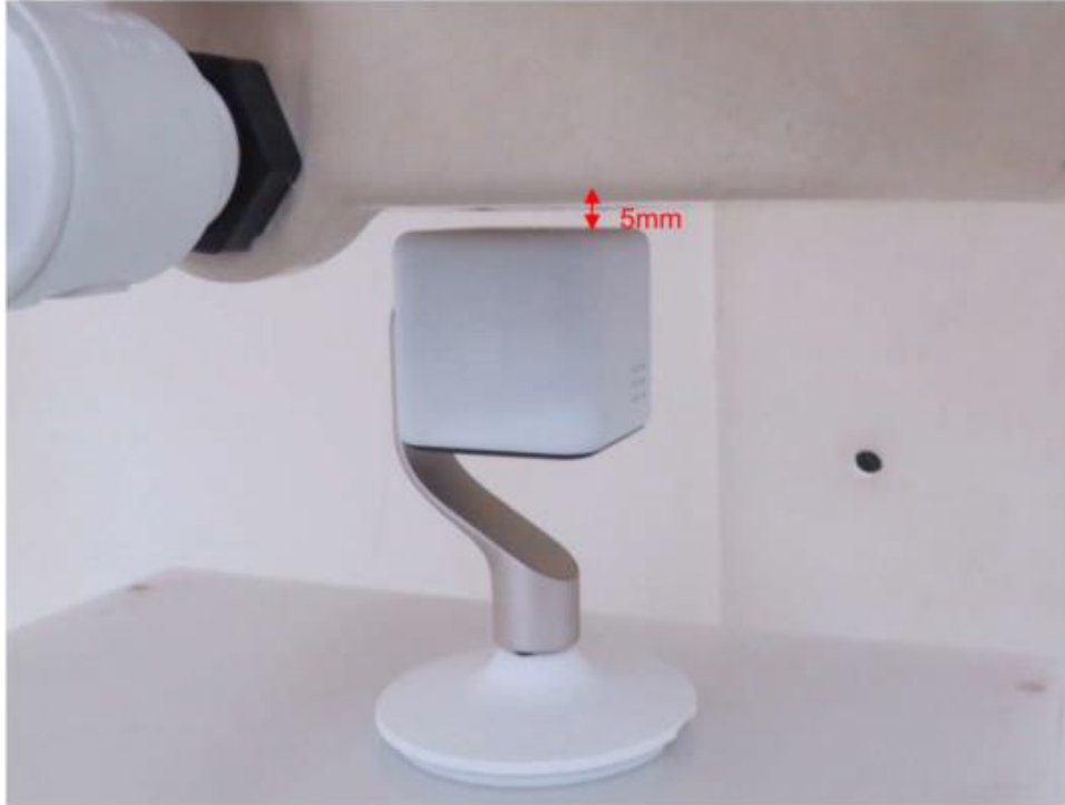
Back side, the distance from EUT to the bottom of the Phantom is 5mm
