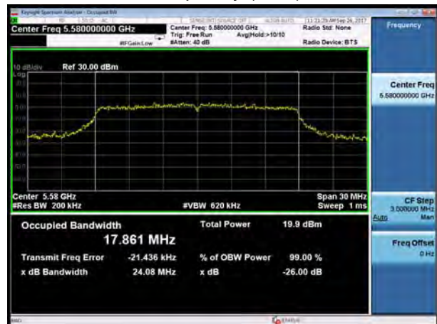
U-NII-2C, 802.11ac HT20 Carrier frequency (MHz): 5700
