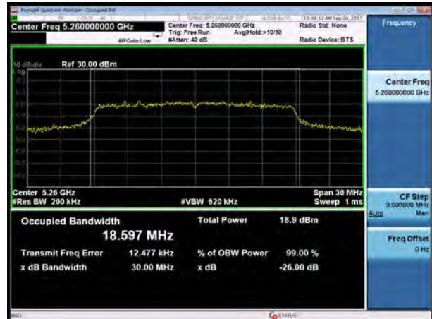
U-NII-2A, 802.11n HT20 Carrier frequency (MHz): 5300
