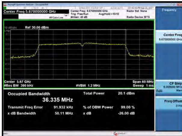
U-NII-2C, 802.11ac HT40 Carrier frequency (MHz): 5550
