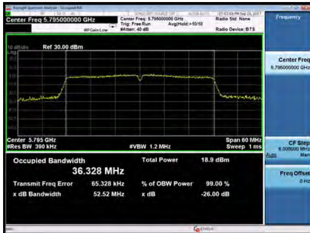
U-NII-3, 802.11ac HT40 Carrier frequency (MHz): 5755
