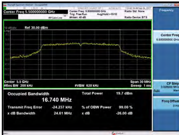
U-NII-2C, 802.11a Carrier frequency (MHz): 5580
