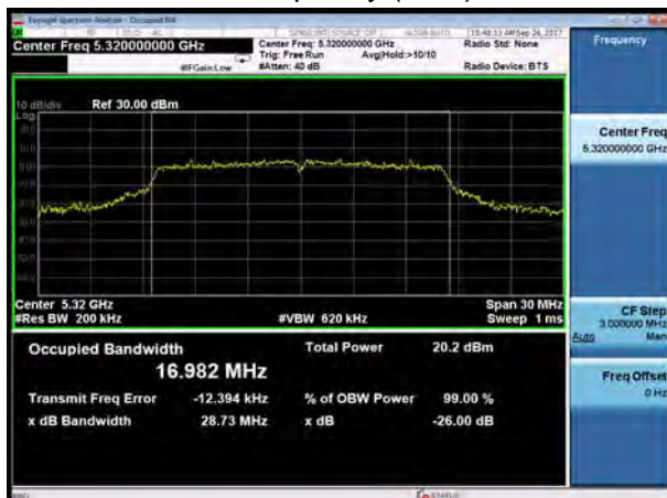
U-NII-2A, 802.11a Carrier frequency (MHz): 5320
