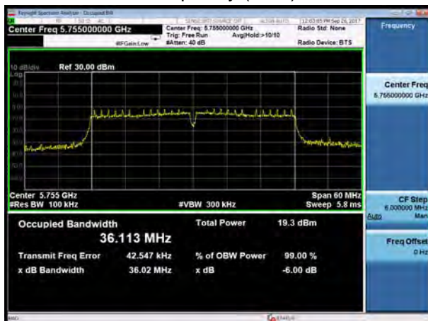
U-NII-3, 802.11ac HT40 Carrier frequency (MHz): 5755
