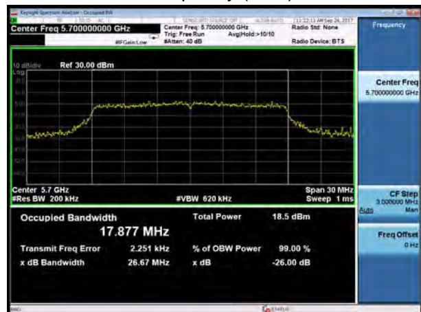
U-NII-2C, 802.11ac HT20 Carrier frequency (MHz): 5700
