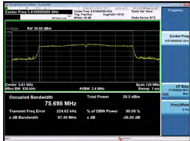
U-NII-2C, 802.11ac HT80 Carrier frequency (MHz): 5610
