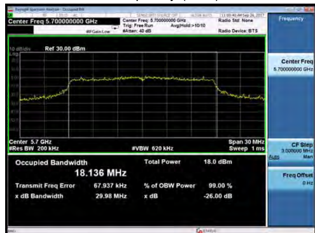
U-NII-2C, 802.11n HT20 Carrier frequency (MHz): 5700
