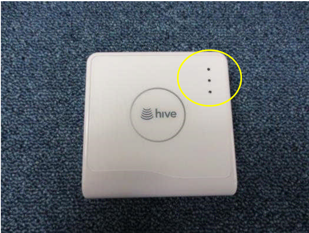
Photograph shows the location of the status LEDs (circled)
