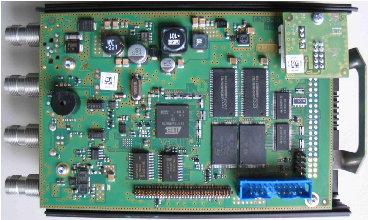
Controller Module mounted
