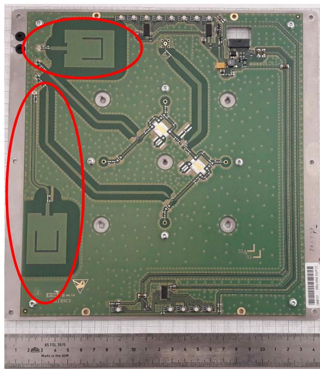
Red marked are the 2 wifi patches with connectors that are connected to the wifi module on main pcb.
