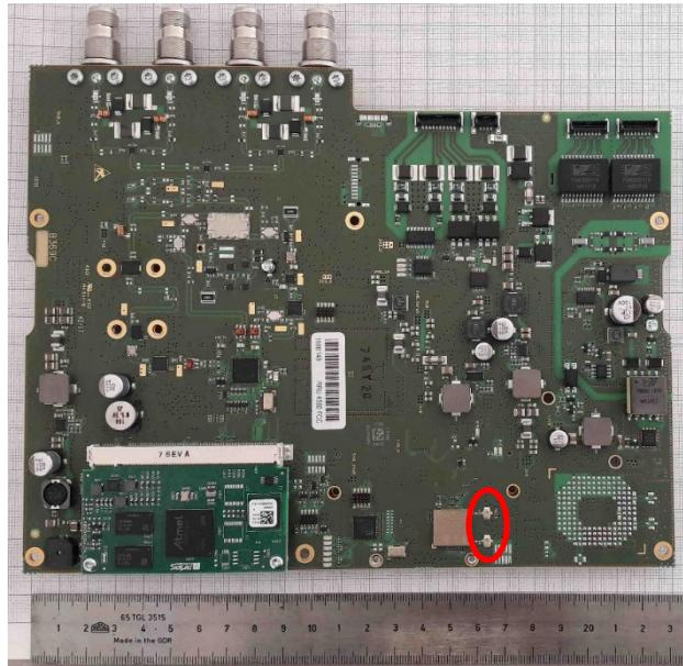
Red marked are the 2 wifi u.FL connectors to be connected to the wifi antenna patches.
