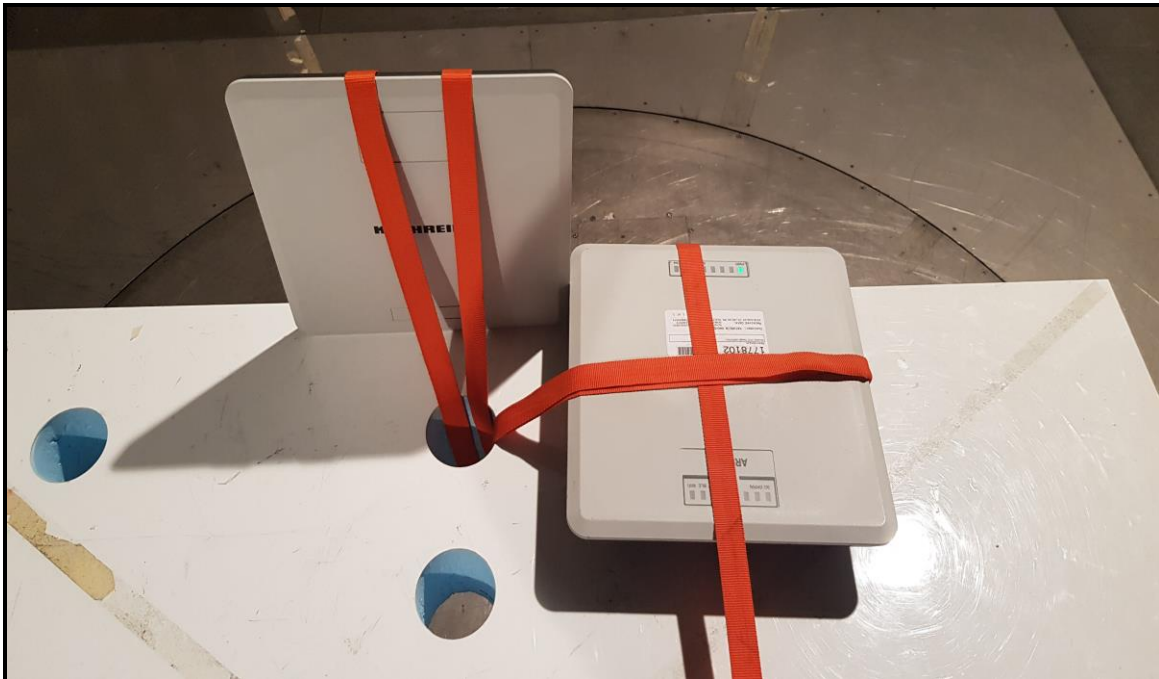
Photo 3: ARU 3560 + WRA 7070 Antenna Unit
