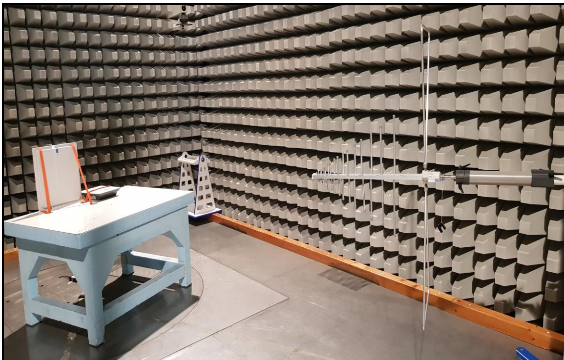
Photo 8: ARU 3560 + WIRA-40-linear-FCC Antenna
