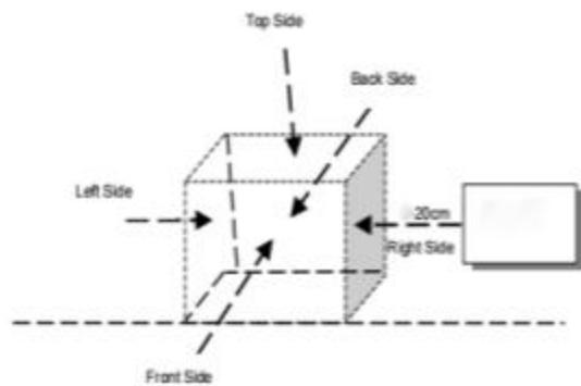
Note: Position A: Front of EUT; Position B: Left of EUT; Position C: back of EUT; Position D: Right of EUT; Position E: Top of EUT(20 cm measure distance);
