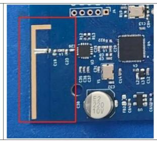
The antenna is PCB antenna. The best case gain of the antenna is 1.54 dBi.
