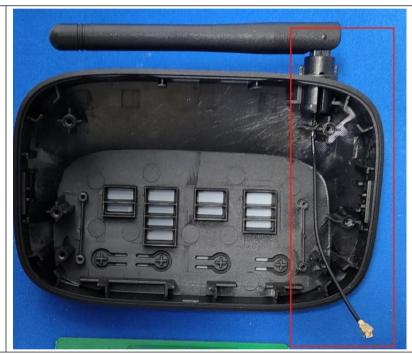
The antenna is Hose antenna. The best case gain of the antenna is 3 dBi.
